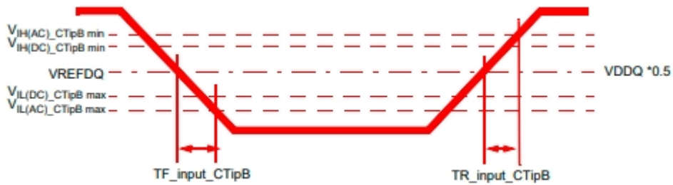
Figure 31 – CS_n and Input A Slew Rate Definition
